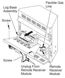
Figure 21 - Removing Log Base Assembly From Fireplace
